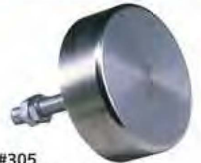
ECS #305 Knob, Anti Slide, St/St. 3" O.D. x 1" High 3/8-16 Threaded Rod 2 1/2" long
