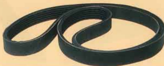
ECS O-G0717A1 Belt, Handrail Pressure, 506 1 \frac{1}{4} " Wide, 98 \frac{1}{2} " Circumference 7 Ribs, Kevlar Reinforced
