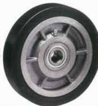
ECS O-A290AB1P Roller, Step or Chain 5½" O.D. x 1½" Tire Face (2) 1½" Bearing I.D. 1 Grease Fitting
