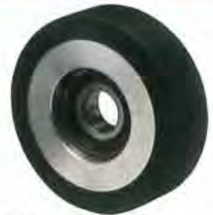
ECS M-P5985 Roller, Step Trail 3 15/16" O.D. x 1 1/4" Tire Face 3/4" Bearing I.D.
