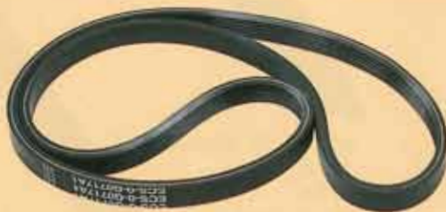
ECS O-G0717A1 Belt, Handrail Pressure, 506 1 \frac{1}{4} " Wide, 98 \frac{1}{2} " Circumference 7 Ribs, Kevlar Reinforced
