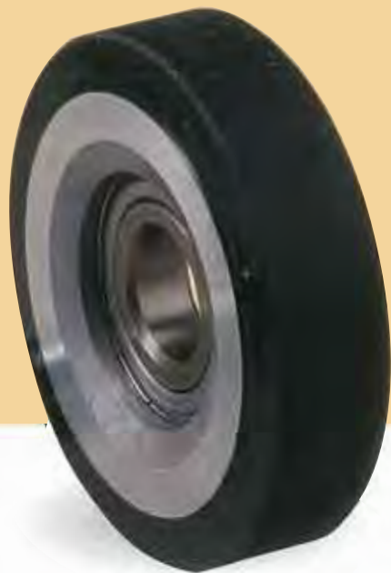
ECS O-290AJ2 Roller, Step or Chain 3" O.D. x 3/4" Tire Face 3/4" Bearing I.D.
