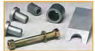
ECS #415 Tool For Removing Worn Brass Bushings From Modular Rack Chain. As It Presses Out The Worn Brass Bushings, It Presses Into Position The New Steel Bushings.
