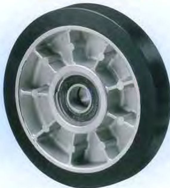
ECS W-217B235H07 Roller, Step Trail And Axle 5 \frac{1}{4} " O.D. x \frac{7}{8} " Tire Face 2 Bearings
