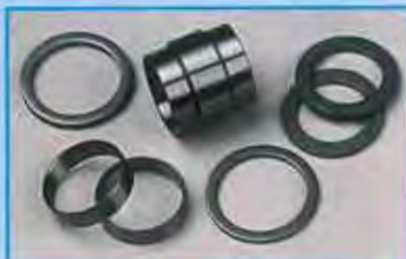
ECS W-6929C24G01 Bushing Kit Needed To Rebush Laminates Having Worn Brass Bushings. 1 1/4" O.D., 2 Kits Per Step.
